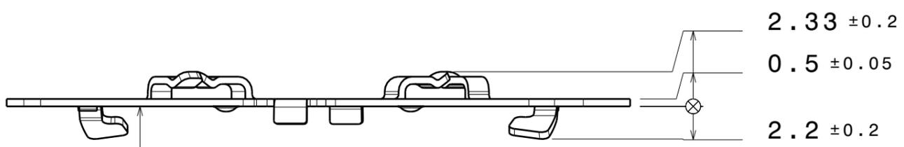
BJB-35-Slim-connector: M3 screw head height max 1.9mm to allow stable assembly result.
